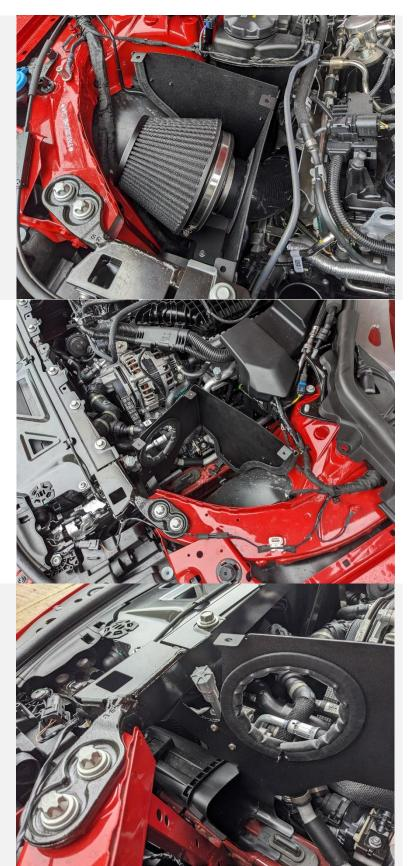
Assemble the front turbo adapter with the other silicone hose and long intake pipe.
