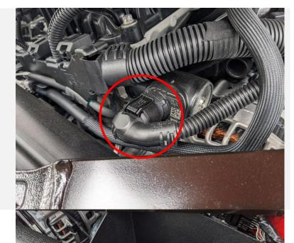
20 Check for clearance around the filters and adjust where need by slackening clamps rotating the silicone.
