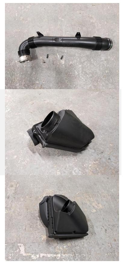
Release the spring clamp securing the right-hand intake hose to the rear turbocharger, and remove the hose. Remove the existing O-rings and spring clamps from the intake hoses. Install them into the supplied adapters. Take note of the orientation of the Orings, it is important that they are installed the correct way round.
